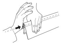
The sealant should overflow all the way round the sealing edge.
